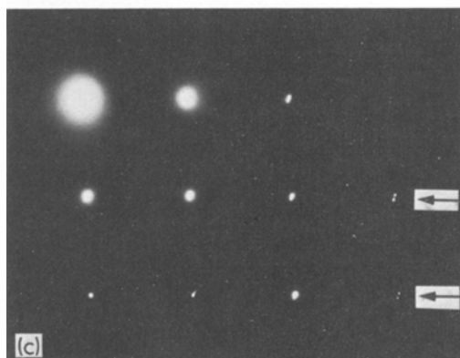
Figure 5 Quenched sample exposed for the first time to the electron beam. Relaxing zig-zag boundary, (b) is taken from the same area a few seconds later; (c) corresponding DP. [0\ 0\ 1] zone (with split spots marked by an arrow).
